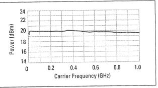
ypical maximum available output power from 0.01 to 1 GHz at 25° C.
