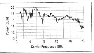
ypical maximum available output power from 1 to 20 GHz, at 25° C vith output step attenuator (Option 1E1) installed.
